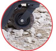
Wide drive and steer wheels-for reduced ground pressure and increased traction on tough job sites.
