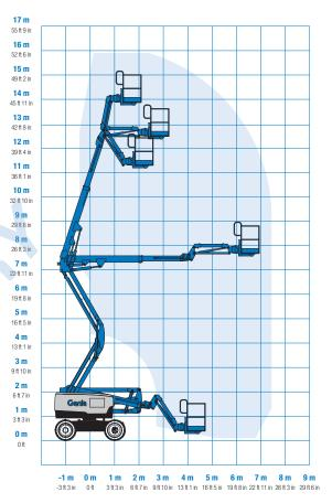
\* The metric equivalent of working height adds 2 m to platform height. U.S. adds 6 ft to platform height. \*\* In lift mode (platform raised), the machine is designed to operate on firm,
