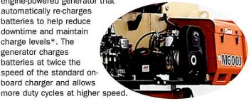
\*Generator can be manually overidden from the platform at any time.
