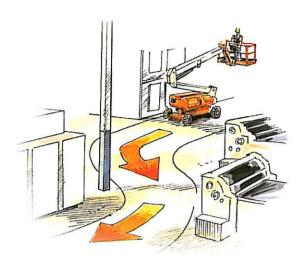
You get over 18 m of high-reach productivity with the added bonus of an electric lift with zero emissions and reduced noise levels - important when working in environmentally sensitive indoor areas. Plus, with a low load bearing pressure of 55 kg and standard non-marking tyres you can drive in areas where care for the floor is an important consideration.
